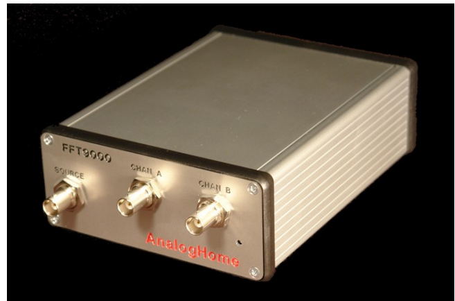
Figure 16 – The experimental Lock-In Amplifier design fits in a 5 x 6 x 2 inch tall commercial enclosure.
